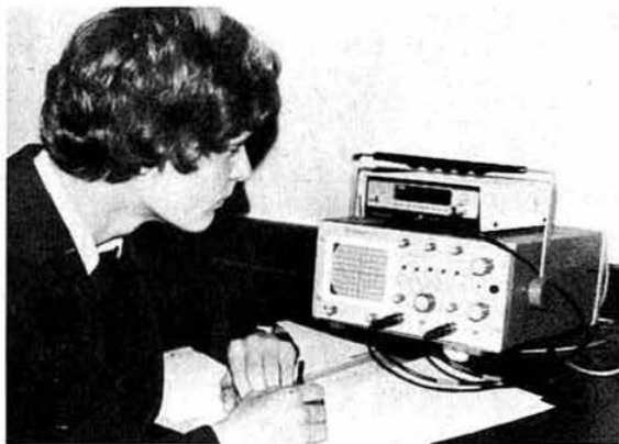
A student measuring doppler shift (suppressed-beam method)
