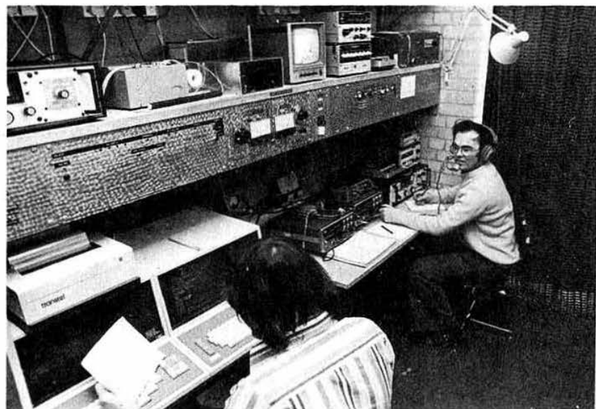
Command centre showing (l to r): autocommand logic, az/el control and Oscar 8 command encoder (in panel); and the on-line facility to the ICL 1905 and (on right) the author at the communication equipment controls
